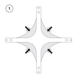
Bend Fig 1 along the fold line downwards. The central part of fig should bend.
