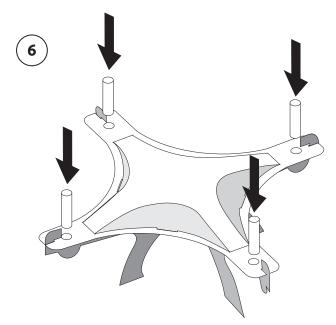
Install the assembled figs 5 (a, b, c and d) into the slots of figs 1-2.
