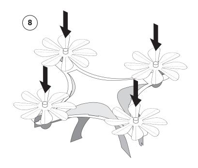
Install the propellers (figs 6) on the tubes (figs 5)
