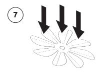
Bend the propeller blades (figs 5 a, b, c and d) along the bend line
