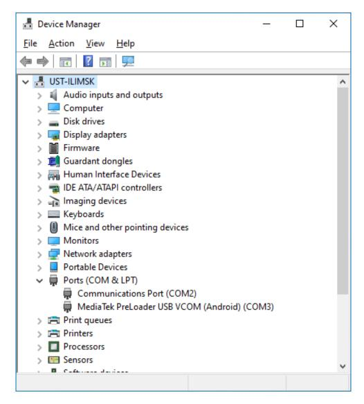
**Confirmation**: Watch out for changes on the **Device Manager** window. After you connect the smartphone to the PC, the **MediaTek PreLoader USB** driver will appear for a short period of time and then disappear.
