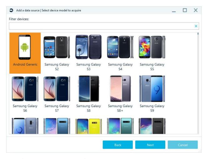
Use the filter to select the device model, if the device model is not shown in the list, select **Android Generic**.
